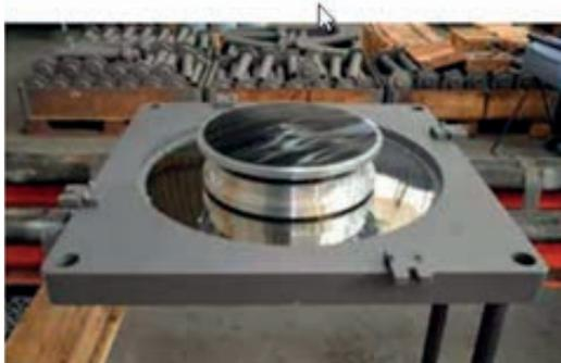
Bottom main sliding surface with articulated slider
